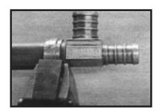
Grasp clamp with tool head and squeeze handles together.
