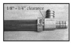
Cut tubing squarely. Slide clamp over tubing. Inswert tubing into fitting. Allow 1/8" to 1/4" clearance between fitting and clamp.
