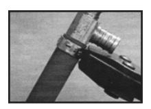
Use the ratchet tool to grasp tab. Pull firmly. The clamp should release.
